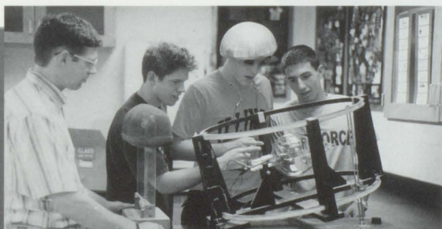
Mr. Norrick observes Greg Crider, Bob Wood, and Starbuck Conyers as they experiment to find the mass of an electron with Helmholtz coils and a Van De Graaff hat.
