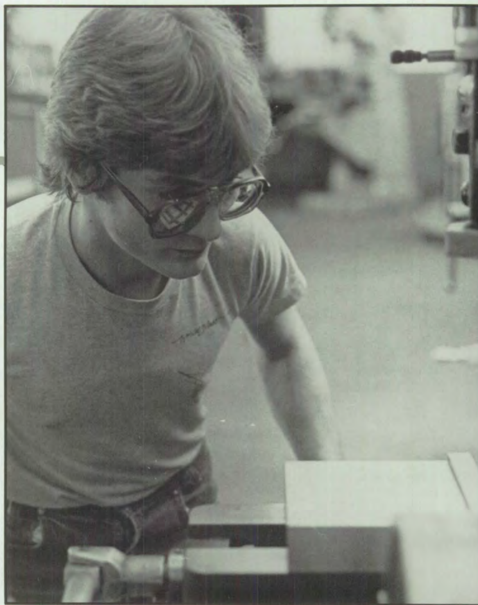
SQUARING IT UP ... Tony Morgan, VICA-Machine Shop student, squares on the vertical mill.
