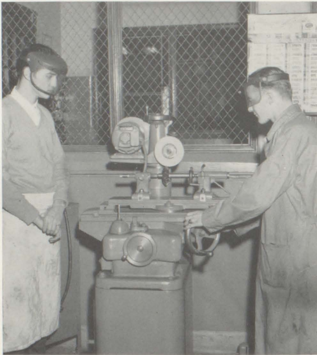
Arnold Hubbs watches Larry Abrell as he starts to sharpen a tool on the tool and cutter grinder.
