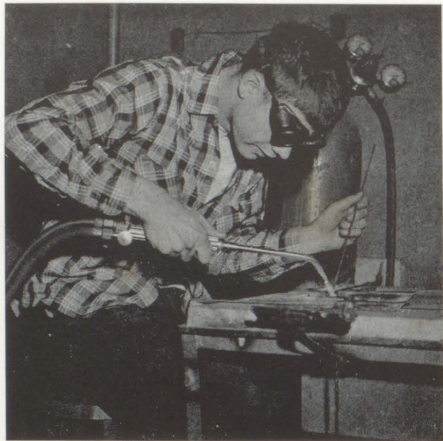
Goggles and torches are standard equipment for Earl Dominick who is learning the fundamentals of welding.
